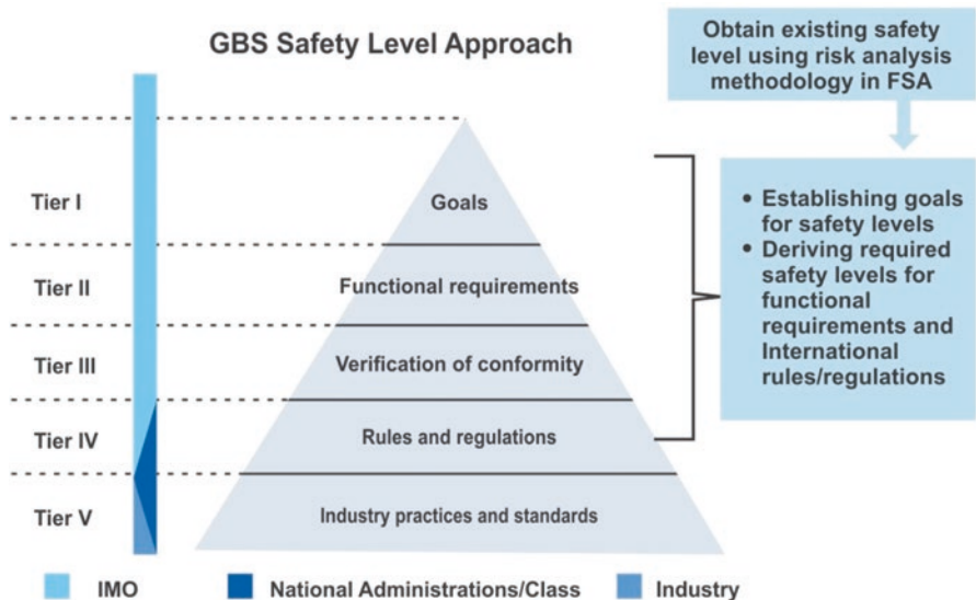
Fig. 12.3 IMO safety case goal-based standards framework (IMO 2019a)
