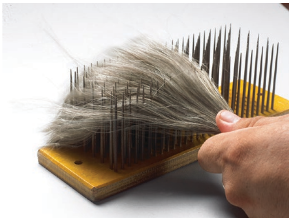
Fig. 19.3 Blending hair to produce uniform tresses of fibers from a range of individuals. (Picture courtesy of International Hair Importers, New York)
