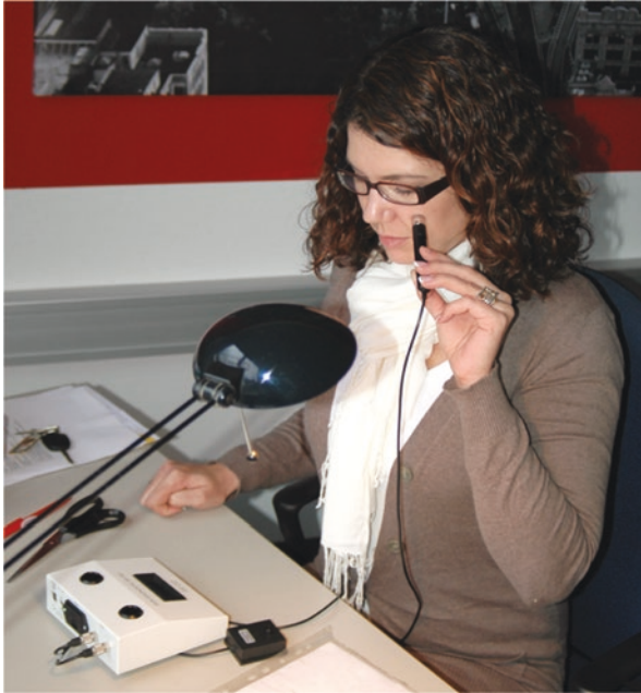
Fig. 26.1 Application of the Corneometer® Mobile Data Collector DC 3000 at the working place of a volunteer on the cheek. Note that an ambient measurement device (temperature, relative humidity) (←) is also attached to the Mobile Data Collector
