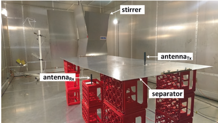
Fig. 6.11 The measurement setup for testing the immunity/performance of LPWAN systems to the multipath phenomenon in the reverberation chamber at WUST ECL
