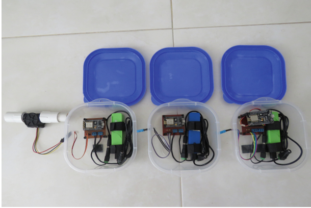
Fig. 2. IoT based irrigation system prototype
