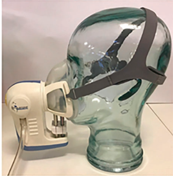
Fig. 6.3 Collection system using ReCIVA device [47]
