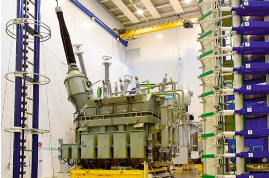
Fig. 8 Synthetic ester immersed transformer for 420 kV class
