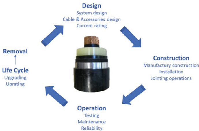
Fig. 1 Life cycle of insulated cables
