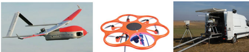
Picture 14 Unmanned aerial vehicles for inspection of OHL. Left: Fixed-wing aircraft, middle: multicopter, right: ground system vehicle for helicopter [6]
