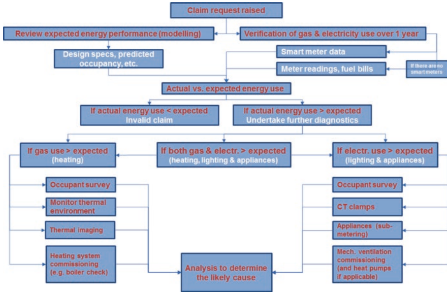
Fig. 1 Methodology flow chart: monitoring and testing protocol in the event of a claim
