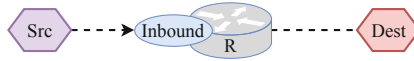
Fig. 1. Routers typically report the address of the interface that received the traceroute probe (inbound address).
