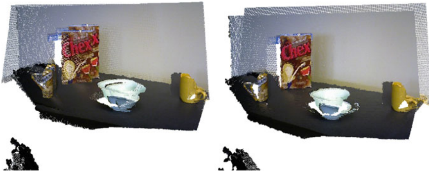
Fig. 8.10 2D Registration: starting views (left) and registered views (right)
