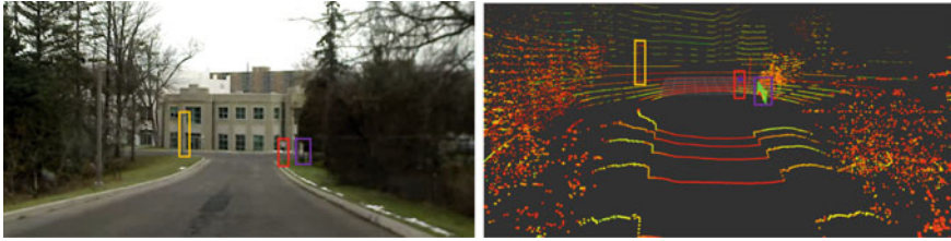
Fig. 4.15 Snapshot of an area using a camera (left) and a view of the same area using VLP-16 LiDAR (right). Note the stop sign, the street sign and the street light pole contained in the red, purple, and yellow rectangles, respectively. Figure courtesy of NRC
