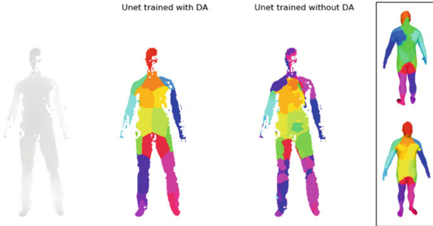
Fig. 5.22 From left to right: actual range image acquired with a temporal encoding structured-light system, where the depth is coded using Gray levels; results of a deep learning approach to human body parts segmentation trained with and without domain-specific data augmentation (DA) strategy that closely simulates the actual acquisition including the system parameters and typical artifacts present in the range images [96, 97]; a reference segmentation provided to qualitatively assess the results of the segmentation. Figure courtesy of NRC
