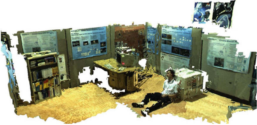
Fig. 2.26 3D model of a mock crime scene obtained with a hand-held stereo camera. Figure courtesy of [78]
