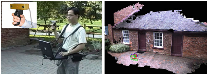
Fig. 2.23 The user points the stereo camera freely at the scene of interest (left), and the photo-realistic 3D model of the scene is generated (right). Figure adapted from [77]
