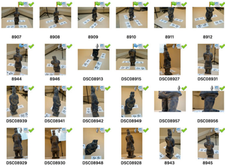
Fig. 13.18 A sample of the images taken for the photogrammetric 3D digitization of the sculpture
