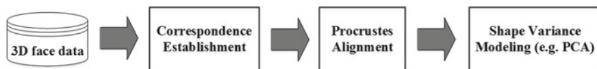
Fig. 10.4 Classical 3DMM modelling pipeline, from 3D face data to the final statistical model
