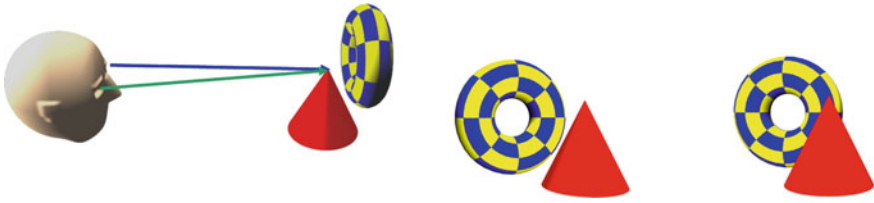
Fig. 1.1 Left: Human binocular perception of 3D scene. Right: the perceived images of the left and right eye, showing how the depth-dependent disparity results in a parallax shift between foreground and background objects. Both observed images are fused into a 3D sensation by the human eye–brain visual system
