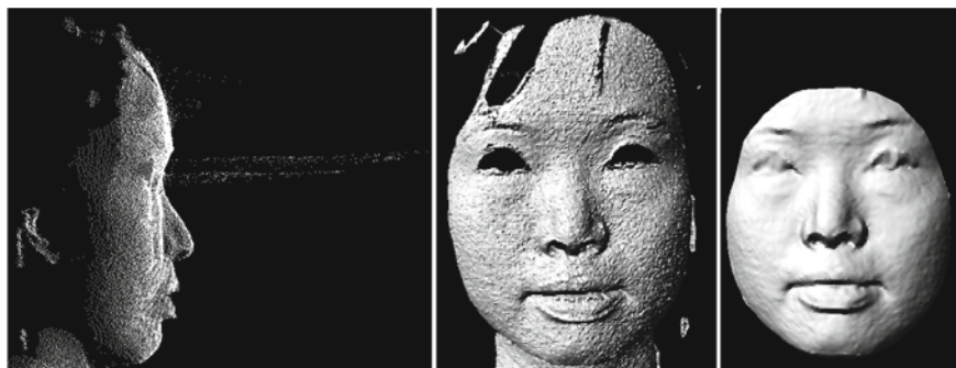
Fig. 12.7 From left to right. A 3D capture of a face with spikes in the point cloud. Shaded view with holes and noise. Final preprocessed 3D data after cropping, removal of spikes, hole filling, and noise removal. Figure courtesy of [70]
