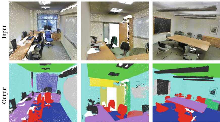
Fig. 11.15 Qualitative results for semantic segmentation. Top row is an input point cloud with color. Bottom row is output semantic segmentation result (on points) displayed in the same camera viewpoint as input
