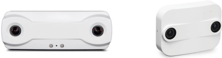
Fig. 2.21 Examples of stereo-based people counters for retail analytics: FLIR Brickstream camera (left) and Xovis PC2 camera (right)
