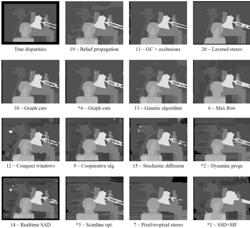
Fig. 2.16 Comparative disparity maps for the top 15 dense stereo matching algorithms in [75] in decreasing order of performance. The top left disparity map is the ground truth. Performance here is measured as the percentage of bad matching pixels in regions where there are no occlusions. This varies from 1.15% in algorithm 19 to 5.23% in algorithm 1. Algorithms marked with a * were implemented by the authors of [75], who present a wider range of algorithms in their publication. Figure courtesy of [75]
