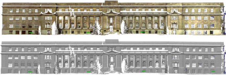
Fig. 4.12 Facade of a building facing south, Top: color from the onboard laser scanner 2D camera mapped onto the final 3D point cloud. Bottom: shaded view of the 3D point cloud. The polygonal mesh was created without using a hole-filling algorithm, using Polyworks IMMerge (no scale provided on this drawing). Figure courtesy of NRC
