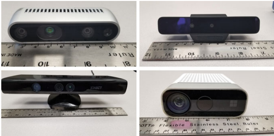
Fig. 5.3 Some of the RGB-D cameras discussed in this chapter. Top-left: Intel RealSense D430 which is based on active stereo. Top-right: Intel RealSense SR300 which is based on time-multiplexed structured-light. Bottom-left: Microsoft Kinect I which is based on spatially encoded structured-light. Bottom-right: Microsoft Kinect Azure based on ToF. Figure courtesy of NRC
