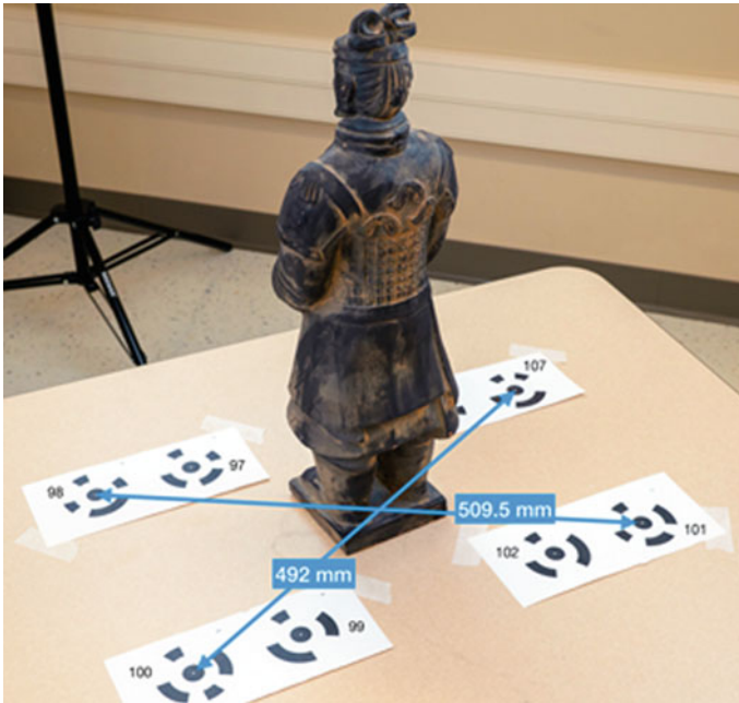
Fig. 13.15 Field preparation before starting the photogrammetric 3D digitization. Two long distances between coded targets are taken with a tape meter for controlling the model scale ( d(100, 107) = 492 mm and d(98, 101) = 509.5 mm), while the shorter distances d(97, 98) , d(99, 100) , d(101, 102) , and d(107, 108) , all equal to 95 mm, are used for checking the scaling result
