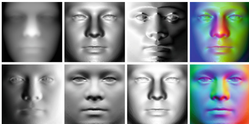
Fig. 12.10 Top row: a range image ( Z values) and its normal maps of elevation \phi and azimuth \theta angles. The three ( Z, \phi, \theta ) values rendered as an RGB image. Bottom row: normal maps of x, y, and z normal components. The three ( X, Y, Z ) values rendered as an RGB image
