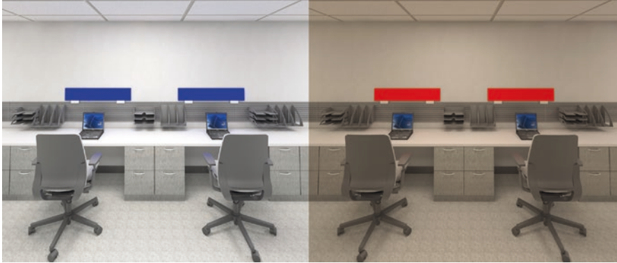
Fig. 15.6 Rendering of a nurses' station during the day shift (left) and night shift (right). High CS to promote circadian entrainment and alertness is provided using higher photopic illuminance levels and saturated blue light from the desktop luminaires during the daytime. Illuminance and CS levels are lower at night, and alertness is promoted by saturated red light that does not affect the circadian system. The same desktop devices, in this case LED light therapy panels, can be configured to deliver both types of light shown here
