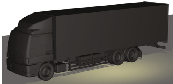
Fig. 15 Truck model. The truck is 12.14 m long, 2.41 m wide, and 3.77 m high
