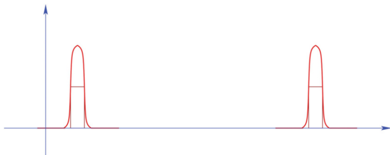
Fig. 6 Two filters to compute two slices of the spectrum that are far apart. Note that eigenvectors associated with two distinct slices need not be orthogonalized against each other
