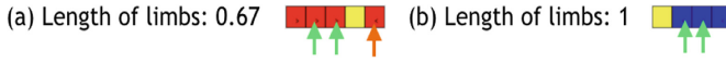
Fig. 4. While in morphology (b) the maximum possible quantity of modules was used as the extension of a limb, in (a), the module indicated by an orange arrow was used as an extra limb. (Color figure online)
