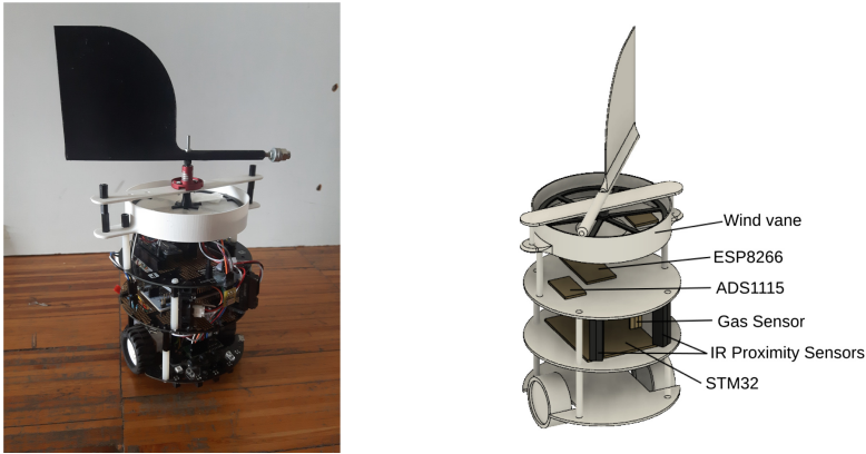
Fig. 2. (Left) developed robot; (right) schematic of the robot.
