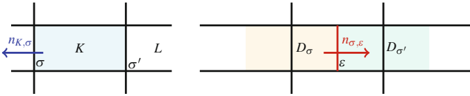
Fig. 1 Notations for control volumes and edges—left: primal mesh, right: dual mesh for the first component of the velocity
