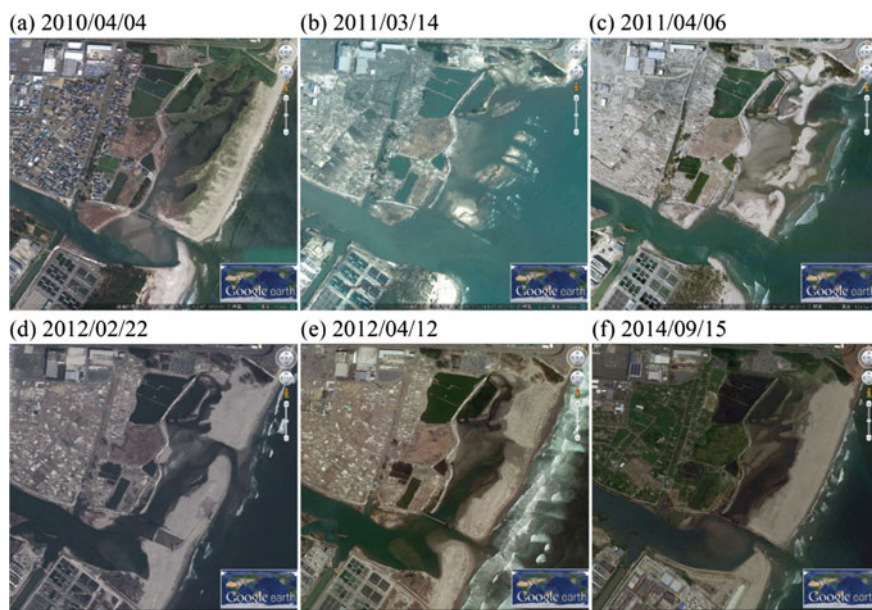
Fig. 2 Topographical changes of Gamo Lagoon before and after the 2011 earthquake and tsunami using Google Earth ( https://www.google.co.jp/intl/ja/earth/ ). a Before the earthquake and tsunami. b Just after the earthquake and tsunami. c Sand deposits were quickly observed. d River mouth was closed and a new water mouth was formed inside the Lagoon. e River mouth was constructed at the previous position. f Present Gamo Lagoon and Nanakita River mouth
