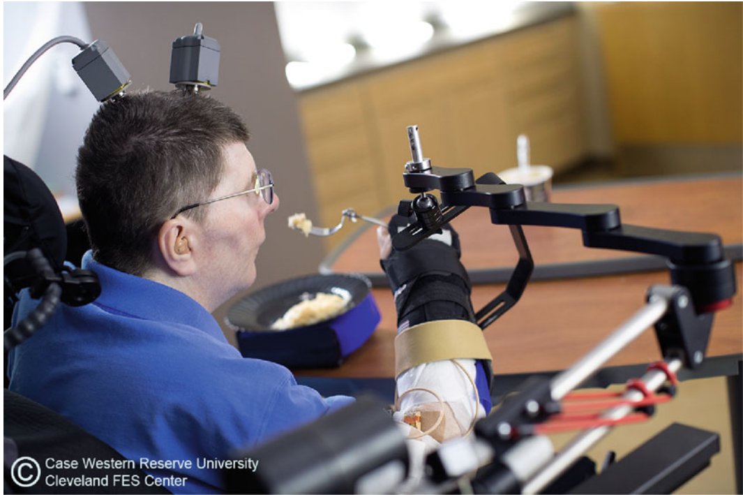
Fig. 5.2 An iBMI user controls functional electrical stimulation of muscles in his arm and hand to feed himself as part of the BrainGate2 clinical trials. (Photo credit: Russell Lee; Case Western Reserve University/Cleveland FES Center)
