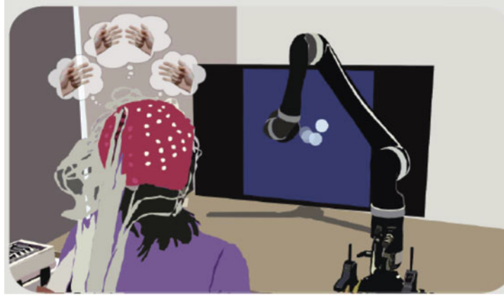
Fig. 4.15 EEG BCI control of a robotic arm in humans. By integrating both the user and machine learning aspects of BCI technology, continuous control of a robotic arm has been demonstrated using EEG source imaged signals.
