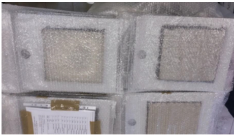
Fig. 3. Special models of the cement-based lining implemented on the steel plates
