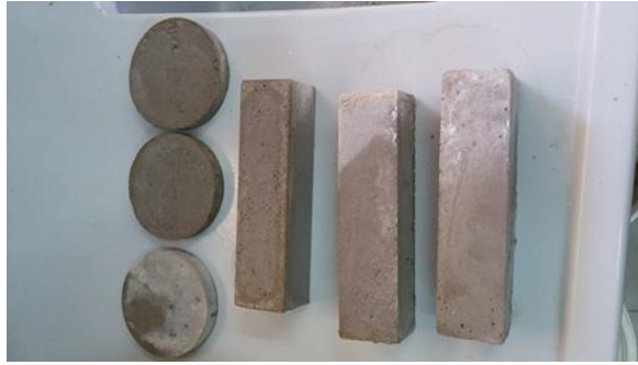
Fig. 1. Samples used in the tests of physical and mechanical properties of hardened mortars
