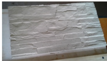
Fig. 2. High performance architectural composite based on dolomite – white cement composition
