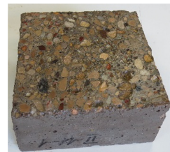
Fig. 3. HP SCC (mix 2) sample after 28 freeze-thaw cycles
