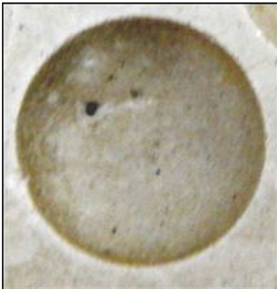
Fig. 2.24 Photographic view of hemispherical cavity on machined workpiece
