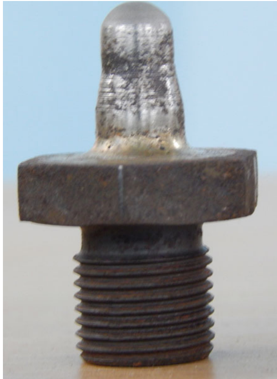
Fig. 2.11 Photographic view of hemispherical tool for USM
