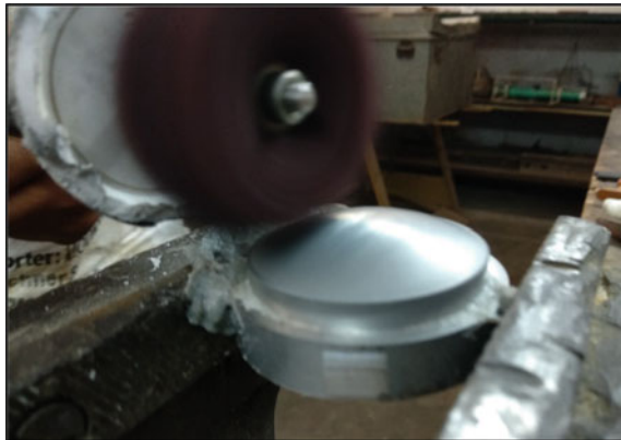
Fig. 11.6 Abrasive float polishing setup used for polishing of curved surface
