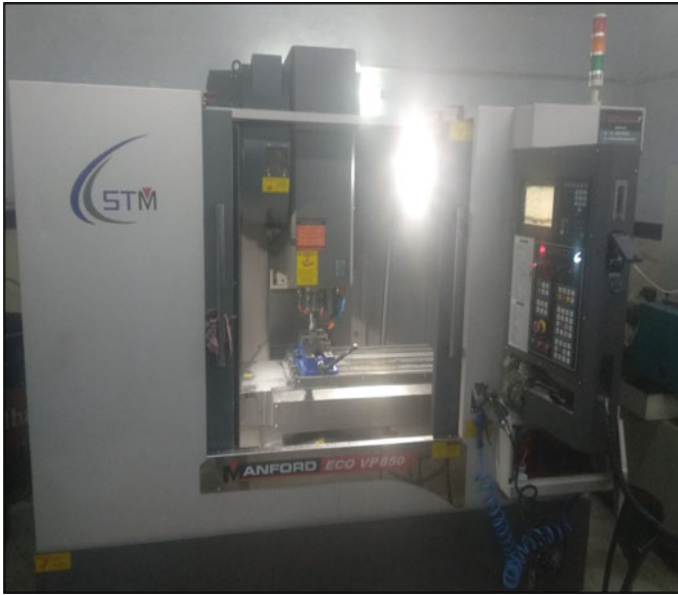
Fig. 11.4 CNC vertical milling centre ANFORDECO VP 850 used for machining of curved surface on Alloy 61S workpiece specimen
