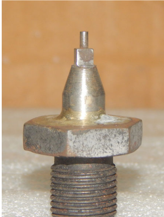
Fig. 2.10 Photographic view of stepped tool having both square and circular cross-section for USM
