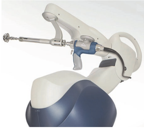
Fig. 31.2 Assembled MAKO acetabular reamer
