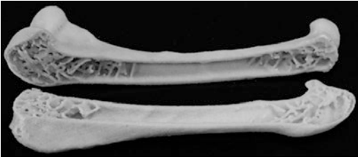
Fig. 35.6 A vertically sectioned femur from a swan which had been imaged with MRI. The bone was segmented out selectively from the DICOM stack and transformed to printable format (stl file) using the free software 3D slicer. The print was rendered using calcium sulfate and binder in the machine shown in Fig. 35.5. Note that the trabecular detail is apparent within the medullary cavity and this internal complexity is not possible to attain by traditional injection molding methods
