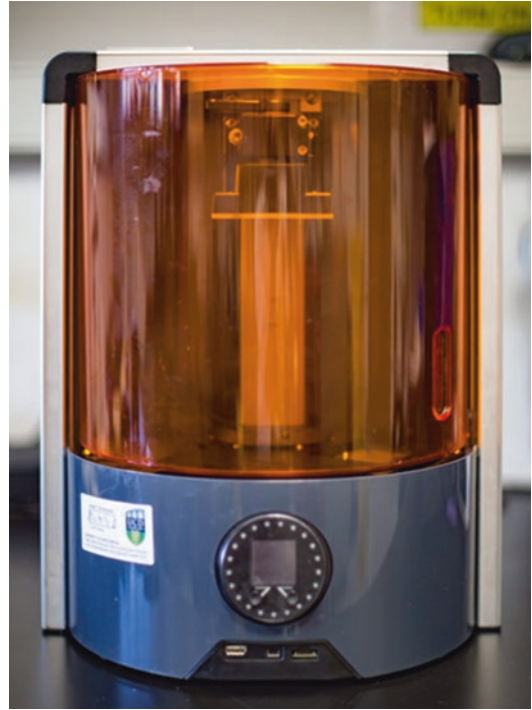
Fig. 35.8 A stereolithography Ember printer which has a 50\ \mu\text{m} spatial resolution in X , Y , and Z directions. This printer uses light to cure photopolymers and results in detailed prints
