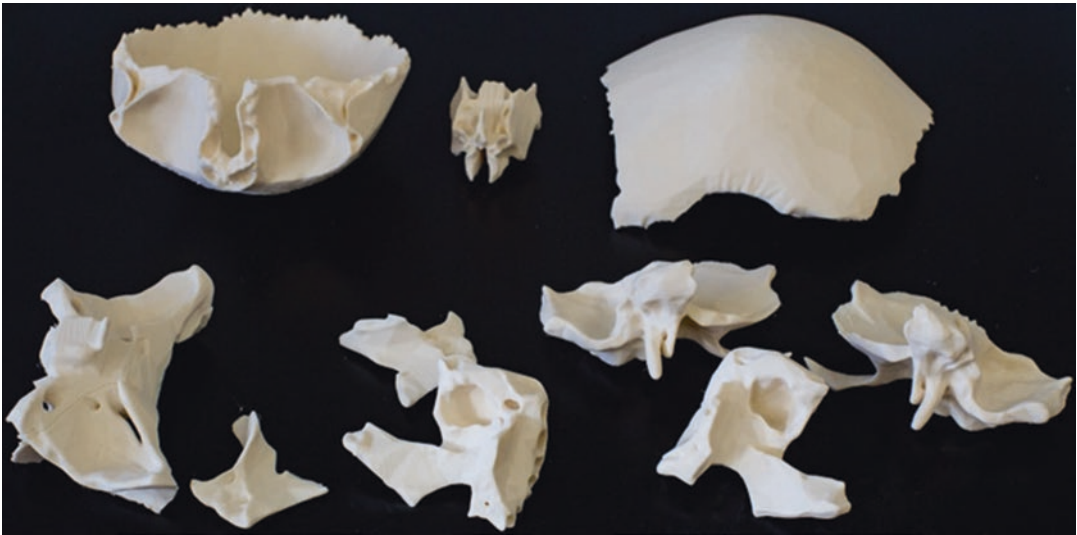
Fig. 35.9 A collection of cranial bones printed with FDM using PLA filament. An ivory-colored PLA filament is superior to white PLA as the resultant prints are more visually realistic. This method augments osteology classes as ethmoidal bones in particular are perishable due to the
