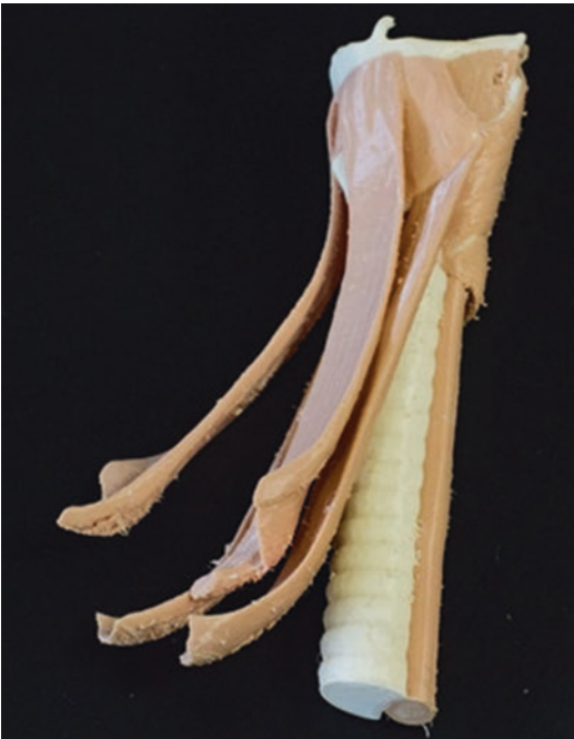
Fig. 35.3 A two-material (flesh Filaflex and ivory PLA) model of upper airway manufactured in a single print. This was created using the machine shown in Fig. 35.2. The cervical strap muscles are very flexible and can be dissected
