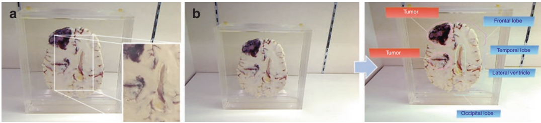
Fig. 34.4 Overview of a tablet AR system using an image marker. (a) Part of the overall cross-sectional image is registered as the marker. (b) An example of how the system works. Left: Plain view of a specimen (not viewed
