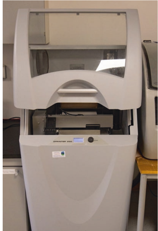
Fig. 35.5 A Z Corp powder binder jetting machine. The parts are supported by powder which does not receive the liquid binder
