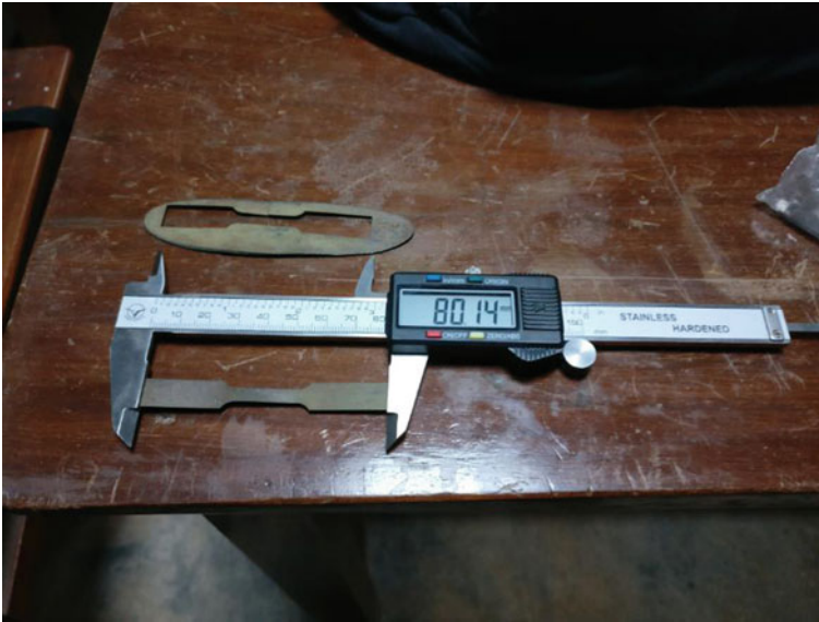
Fig. 7 Actual TiNi specimen cut by wire-EDM
