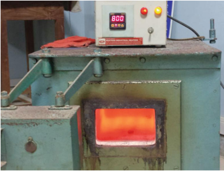
Fig. 3 Furnace used while hot rolling of TiNi alloy
