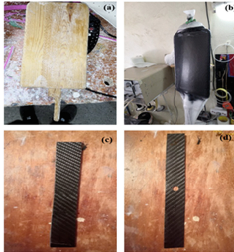
Fig. 1. Specimen preparation (a) wooden mold, (b) final composite product, (c) specimen without hole, (d) specimen with hole
