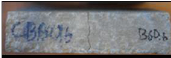
c) Legible crack after tests (WSC).
