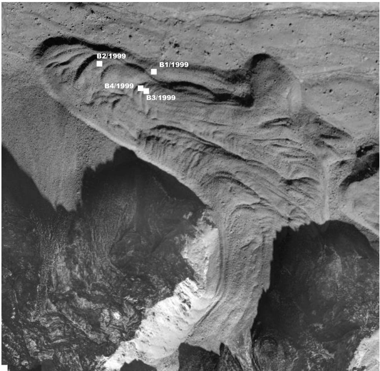
Fig. 16.9 Aerial image (Airborne Digital Sensor) of the Muragl rockglacier showing the surface structure of ridges and furrows as well as the outbreaking lobe to the north (source Swisstopo, PERMOS,
