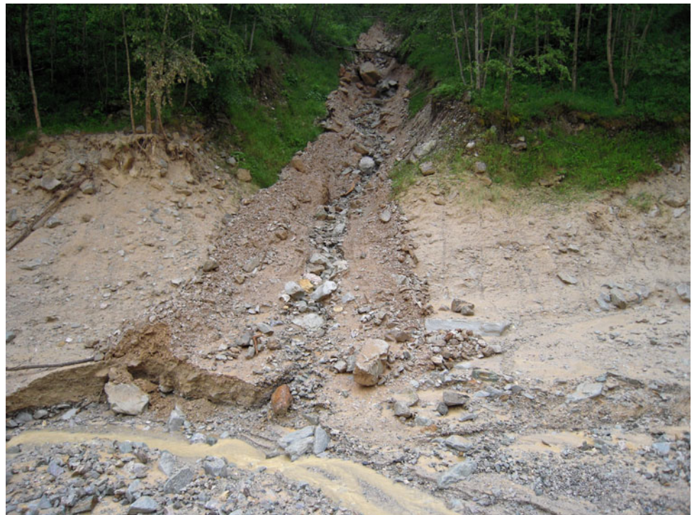
Fig. 25.9 Debris-flow levees at a tributary to the main Illgraben channel (levee spacing is \sim 3 m) (photo B. McArdell)
