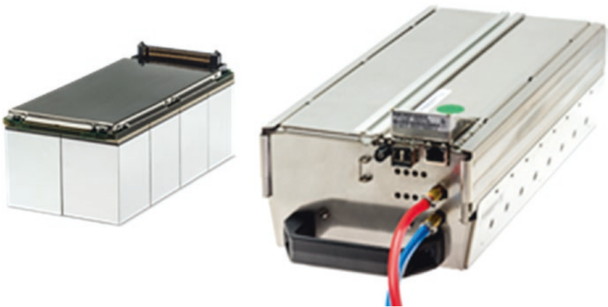
Fig. 6.2 Left, the detector with SiPM. Right, a detector electronics assembly containing 16 detectors and associated electronics
