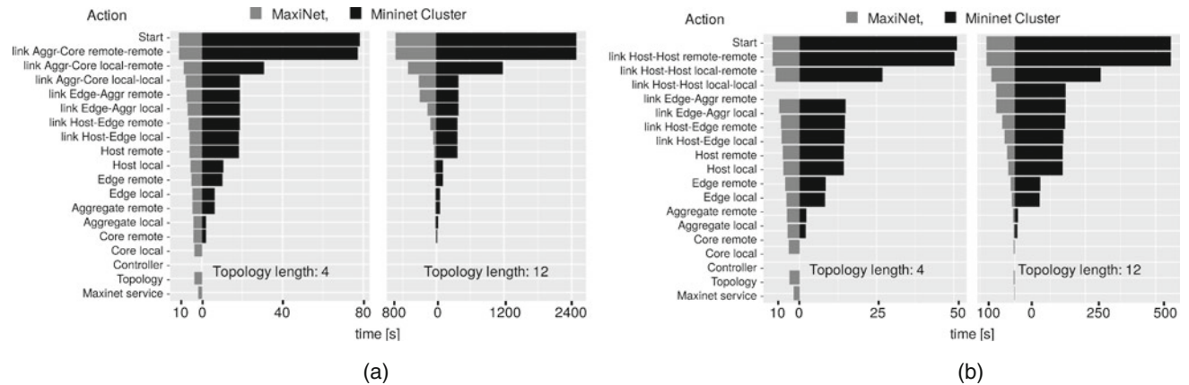
Fig. 77.6 Time taken per setup action in distributed Mininet solution evaluation. (a) FatTree topology. (b) DCell topology
