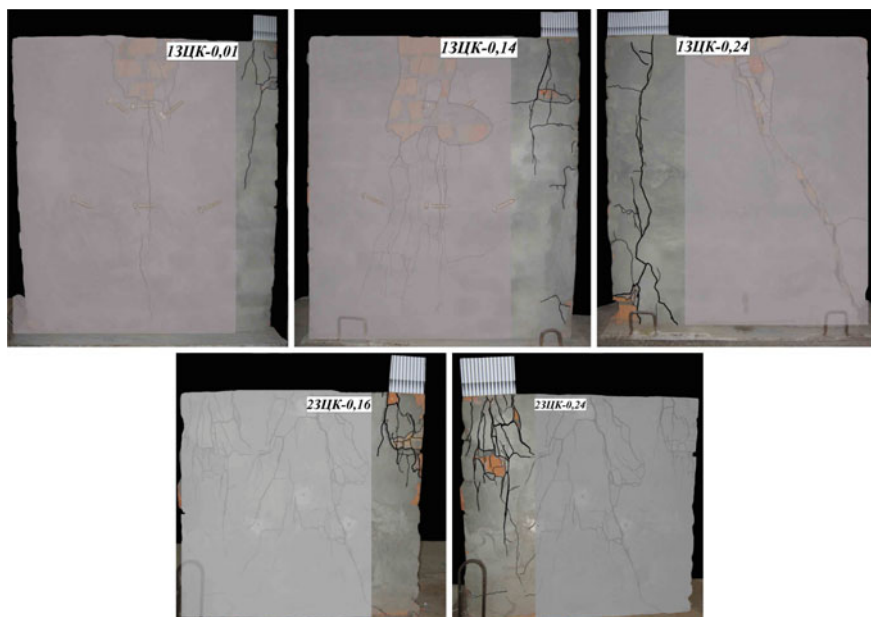
Fig. 6 Nature of the masonry specimens destruction under edge local compression
