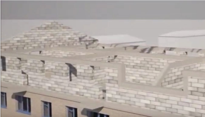
Fig. 7 Reconstruction of the building with an additional storey with lightweight aerated concrete blocks
