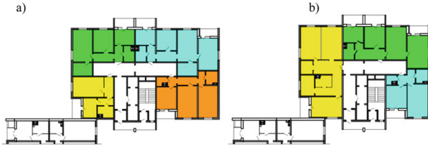
Fig. 5 Planning of the meridional sections: a the existing plan and b a new plan
