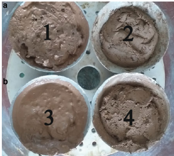
Fig. 2 Type of soil samples of the mixture of drilling waste (a) and loam loess refractory (b) in proportion (a:b),%: 1–70:30; 2–50:50; 3–80:20; 4–60:40
