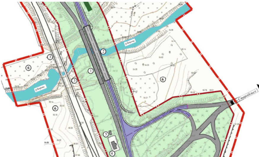
Fig. 2 Detailed plan of the bridge over the Borova River: 1—motorway bridge; 2—perspective bridge; 3—railway bridges; 4—commercial pavilion and summer terrace; 5—car repair shop (tire shop); 6—agricultural reserve areas
