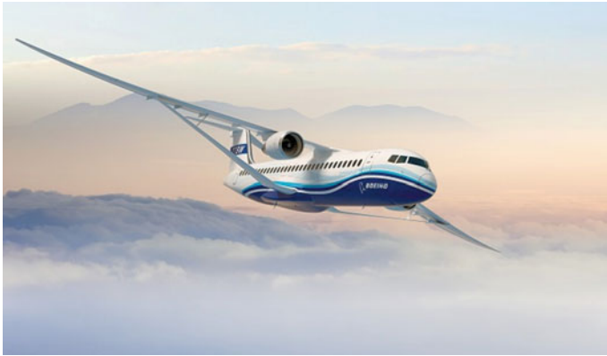
Fig. 2 Combined truss in aircraft construction: lightweight, resilient, ultra-thin sloping wing supports—Boeing and NASA, USA
