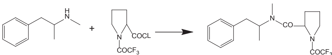
Fig. 12.7 Chiral derivatization of methamphetamine using L -TPC
