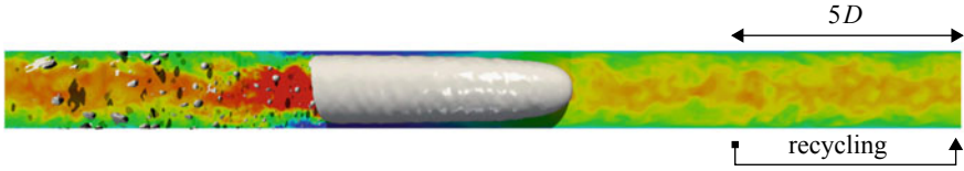
Fig. 18.1 Iso-surface of the instantaneous void fraction at 0.5. Color indicates the axial velocity component in the MFR
