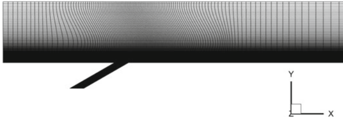
Fig. 8.1 Grid consists in about 542 mln grid points. Here it is shown in the symmetry plane and, for the sake of clarity, only one on eight points is plotted in all the dimensions. A grid clustering is performed in the y - and x -directions
