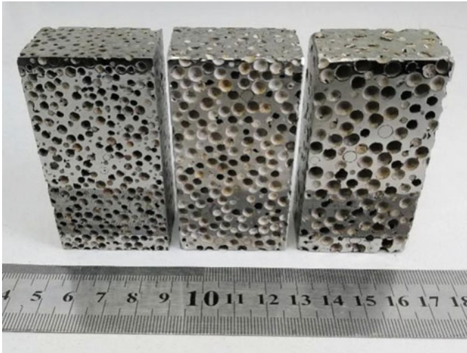
Fig. 4 The samples of steel matrix syntactic foams
