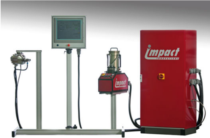
Fig. 3 Upstream injection cold spray system 5/8 (34 KW/50 bar/800 °C) showing control unit, and powder feeder, with a 34 KW gun-mounted gas heater. Photo courtesy of Impact Innovations [5]
