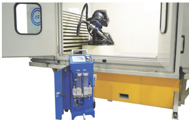
Fig. 9 SST PX downstream injection robotic system (4.2 KW/17 bar/550 °C) integrated with the new dual-non-pressurized powder feeder. Photo courtesy of CenterLine (Windsor) Limited
