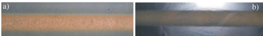
Fig. 11 Macrograph top view of the cold sprayed spherical copper particles onto PC/ABS substrates; the gas pressure was set to 5 bar (a) and 30 bar (b)
