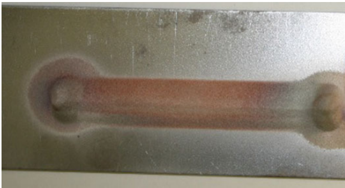
Fig. 6 CuAlNi SMA fabricated by cold spray deposition
