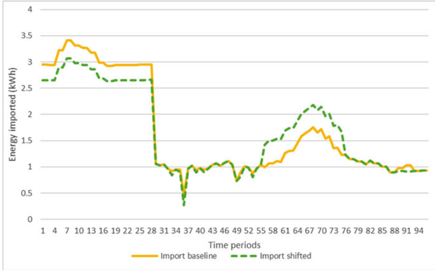
Fig. 4.13 Carrying out a load shifting request
