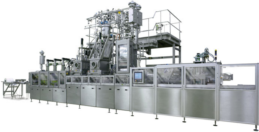
Fig. 25.5 Bosch TFA 4830 aseptic thermoform-fill-seal cup machine. (Courtesy of Robert Bosch Packaging Technology GmbH)
