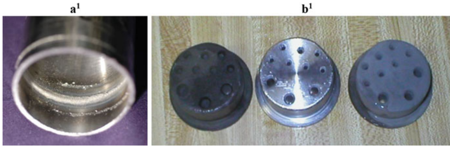
Fig. 12.10 Consequences of improper passivation (Miller 2012). (a) Corrosion from prolonged contact with passivating solution; (b) Material not compatible with passivating solution
