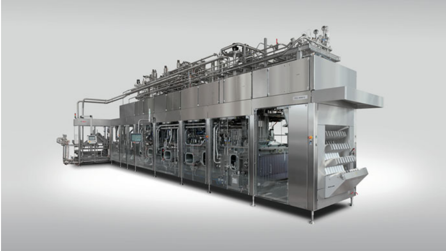
Fig. 25.4 Ampack FCL aseptic fill-seal machine for preformed cup. (Courtesy of Robert Bosch Packaging Technology GmbH)
