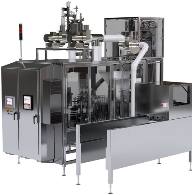
Fig. 25.6 Scholle aseptic fill-seal machine and preformed pouch. (Courtesy of Scholle IPN)
