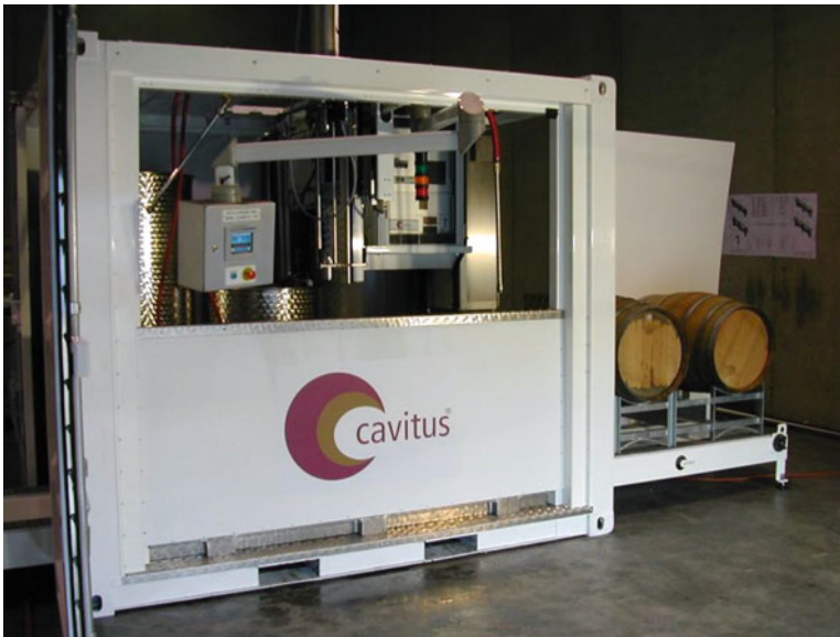
Fig. 22.8 An automatic oak wine barrel cleaning system using a 4 kW ultrasonic transducer (Cavitus Pty Ltd.)
