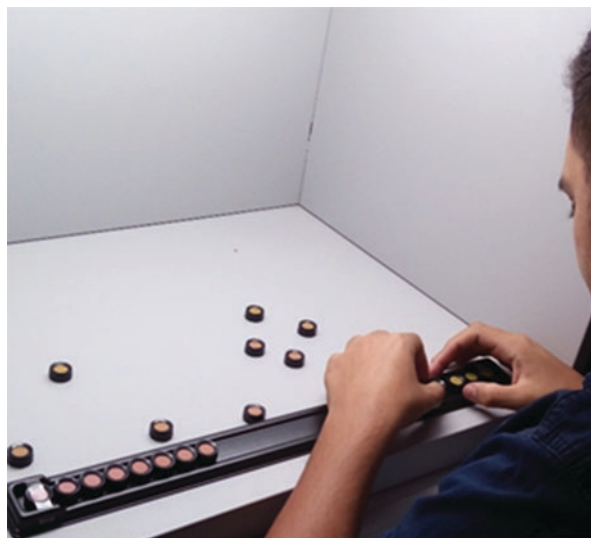
Fig. 6.4 Observer taking the Farnsworth Munsell 100 Hue test under controlled conditions (light or viewing booth)
