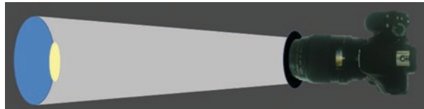
Fig. 5.2 Schematic image of a ring flash with light reflections generated from curved surfaces such as the buccal surface of upper anterior teeth
