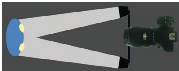
Fig. 5.3 Schematic image of a twin flash on a bracket arm with light reflections generated from curved surfaces such as the buccal surface of upper anterior teeth
