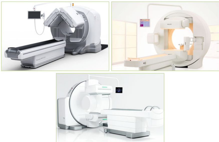
Fig. 17.3 Examples of SPECT/CT Systems. Image adapted from [123]. Upper left—GE Discovery NM/CT 670, two gamma camera heads here configured at 90° combined with a CT System. Upper right—Philips BrightView XCT, two gamma camera heads with a flat-panel detector. Lower image—Siemens Intevo, two gamma camera heads combined with a CT system
