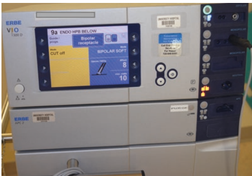
Fig. 22.2 Preprogrammed settings on an Erbe VIO 300D electrocautery generator (Erbe USA, Marietta, GA, USA)
