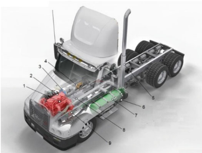
Fig. 44 Structure of a dedicated truck specially designed to work with LNG: 1—fuel injection system; 2—ICE; 3—electronic control module; 4—battery; 5—exhausting system; 6—fuel filter; 7—fuel container; 8—transmission; 9—fuel pipeline
