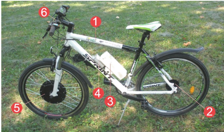
Fig. 13 General view of the electric bicycle: 1—frame; 2—back wheel with a chain mechanism; 3—battery; 4—controller; 5—electric motor; 6—handlebar
