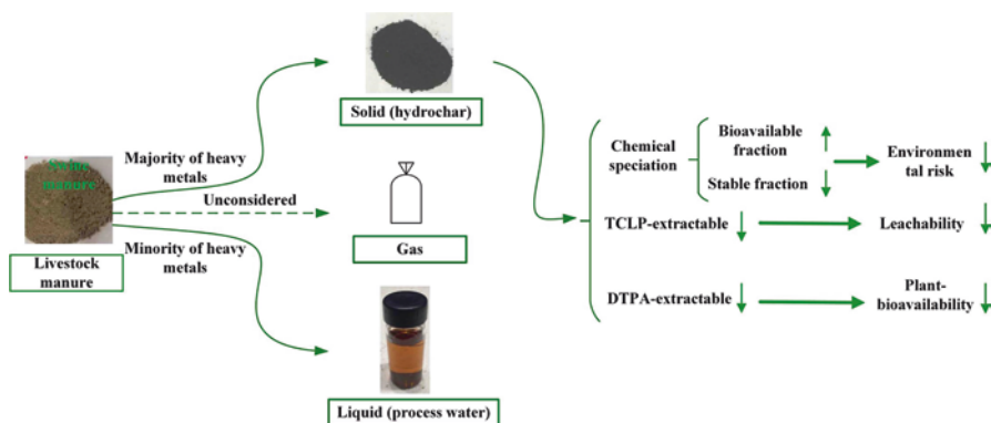
Fig. 7.11 The migration/transformation behaviors of heavy metals during the hydrothermal carbonization of livestock manure
