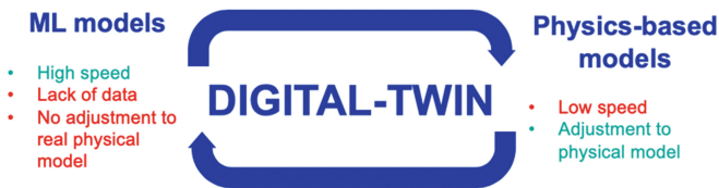
Fig. 2. Digital twin as a combination of data-driven and physics-based models
