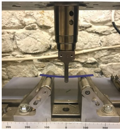
Fig. 6. Three-point bend with tensile machine SHIMADZU
