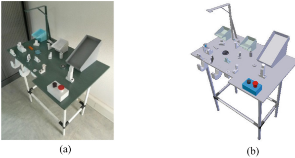
Fig. 1. The Finishing table : (a) the physical prototype and (b) its digital mock-up.
