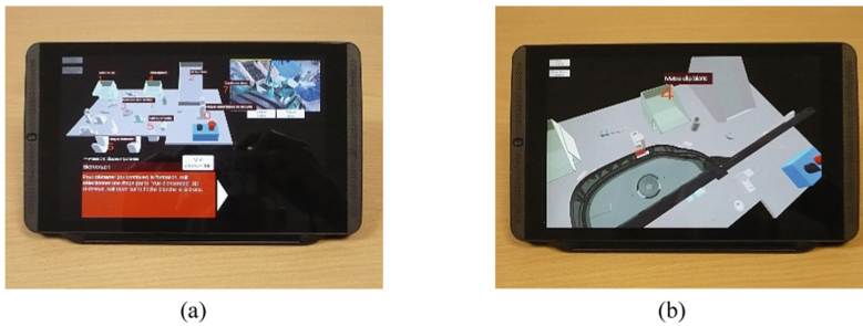
Fig. 3. Tablet prototype: (a) Initial training screen. Note the decomposition of the UI in dedicated zones for animations, videos, textual instructions, and additional images, (b) full-screen 3D view, which can be manipulated freely.
