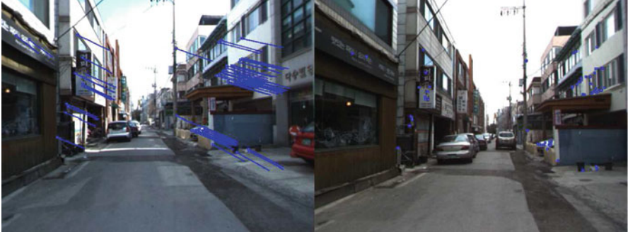
Fig. 11 Corner matching results between the third key-frame image and the last image for calculating final pose errors
