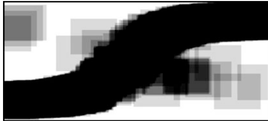
Fig. 8 Overview of image processing. Each point on a sound map replaced with a translucent rectangle. The rectangles overlap and generate a bold line for S-curves that indicate vehicle passing
