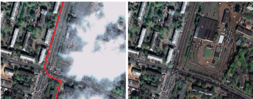
Fig. 9 Orthorectified images obtained by the monotonic direction field algorithm: without cloud removing (left) and with it (right), to obtain the right image the mask of clouds was used (the red line in the left image its boundary). This mask also include some areas near clouds to save integrity of objects (houses and roads)
