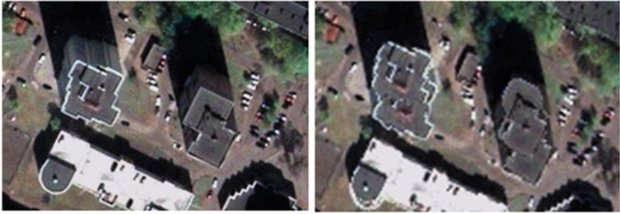
Fig. 3 Satellite image (left) and duplicated buildings (right) in the result of RPC-based orthorectification
