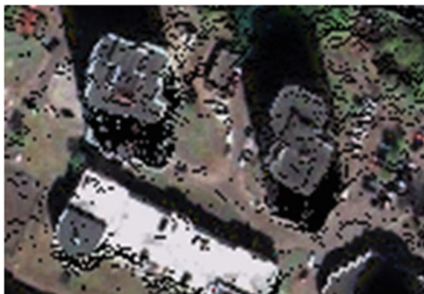
Fig. 5 Overlapped areas (black) obtained by the neighborhood method; it can be seen that the black points are present even on the flat surfaces
