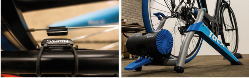
Fig. 4. The reed switch and magnet used to detect the rotational speed of the bike wheel (left) and the bike trainer used to provide resistance (right).
