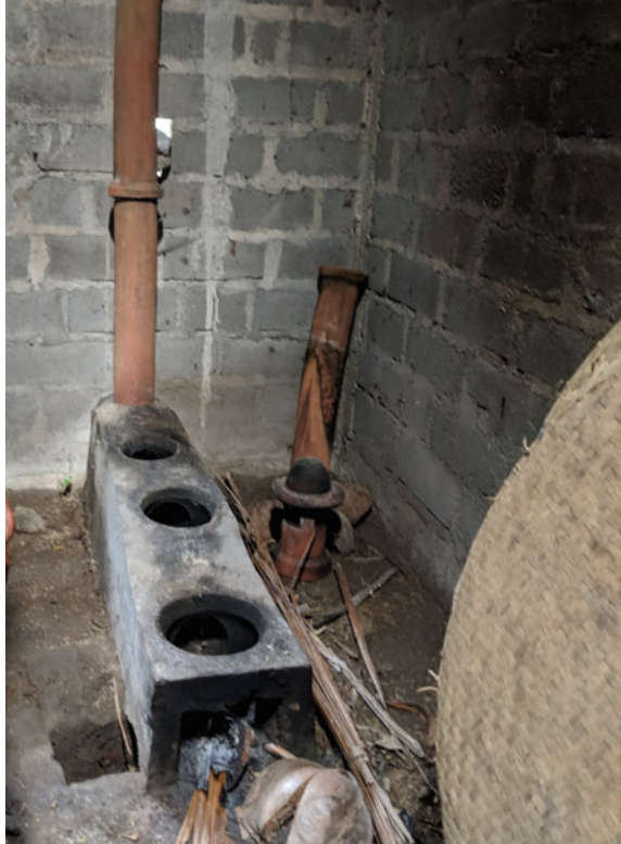
Fig. 3 Traditional chimney-installed cookstove in Yogyakarta area, Indonesia. Source Masak Bersih
