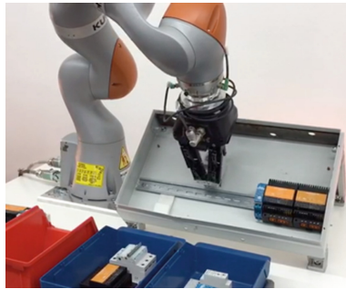
Fig. 1. Automated electrical component assembly by robot
