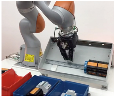
Fig. 1. Automated electrical component assembly by robot
