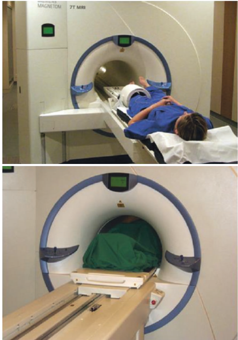
Fig. 4.1 7-T MR scanner with a bore of 60 cm and a length of 3.50 m. The MR is surrounded by 425 tonnes of steel. The upper figure shows a person before positioned feet first into the scanner. The lower figure shows a person head first in the scanner with the head in the isocentre, the feet covered with a sheet. The scanner used here is located at the Erwin L. Hahn Institut, Essen, Germany
